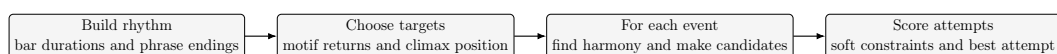
Figure 5.3.3: The melody-generation stage in the third iteration. The generator first decides structural targets, then evaluates candidate notes under the active harmonic and formal context.
